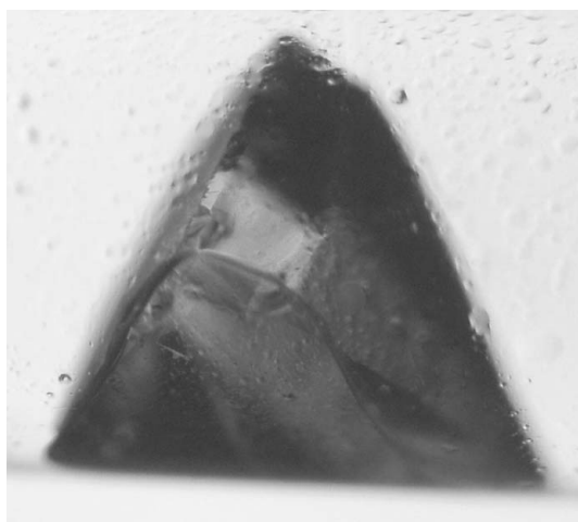
Figure 1 Photograph of the \gamma -chymotrypsin crystal used for this neutron diffraction study on the LADI-III beamline at the ILL. The crystal volume is approximately 1.3 mm 3 .
